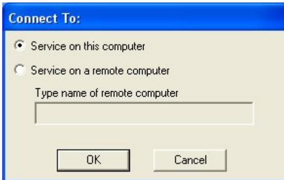
If you are currently on the computer designated as the messaging server, select “Service on this computer:” If you are running the Service Controller on another computer on the network, select “Service on a remote computer” and enter the name of the messaging server computer.
